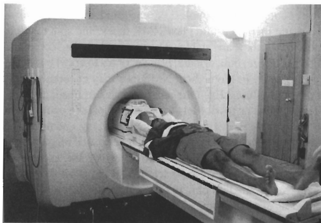
Figure 16.1. A 1.5-T, 100-cm-diameter bore NMR system for human clinical use. The table automatically moves the subject into the magnet.
